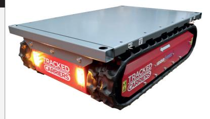
The 1200 series from Dewsbury & Proud the ideal all-round carrier. At just 750mm wide the 1200 R can fit through most doorways, and with a substantial 1,200kg maximum capacity the uses are endless. R models use state-of-the-art technology whilst being simple to operate, reliable and easy to maintain.
